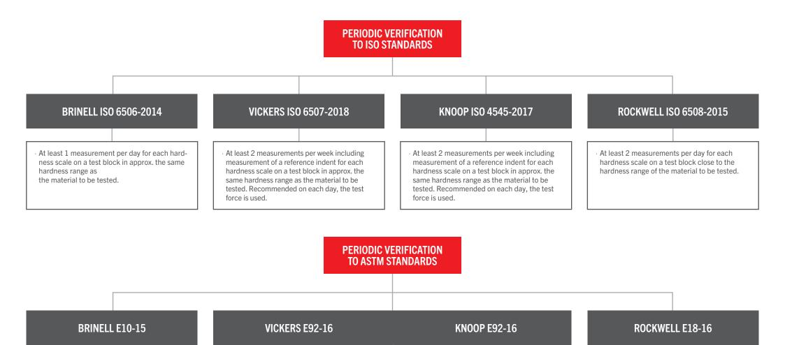
• At least 2 measurements per day on a test block in the hardness range of the material to be tested. • At least 2 measurements per day on a test block in the hardness range of the material to be tested.
