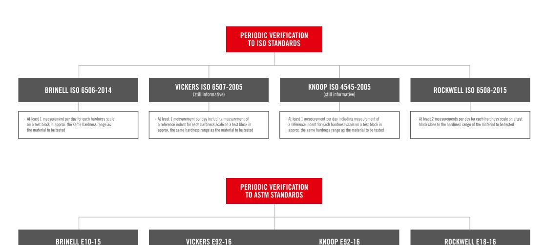
· At least 2 measurements per day on a test block in the hardness range of the material to be tested
